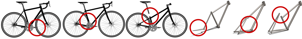
Figure 4: Bike-bench features numerous closed-form constraint checks to identify common geometric infeasibilities such as disconnected or colliding components (left 3). Less common infeasibilities in frame geometry are flagged if the design causes errors during 3D reconstruction (right 3).
