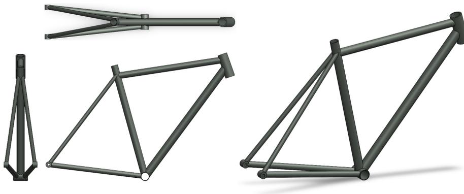
Figure 2: Different views of example bicycle frame model.
